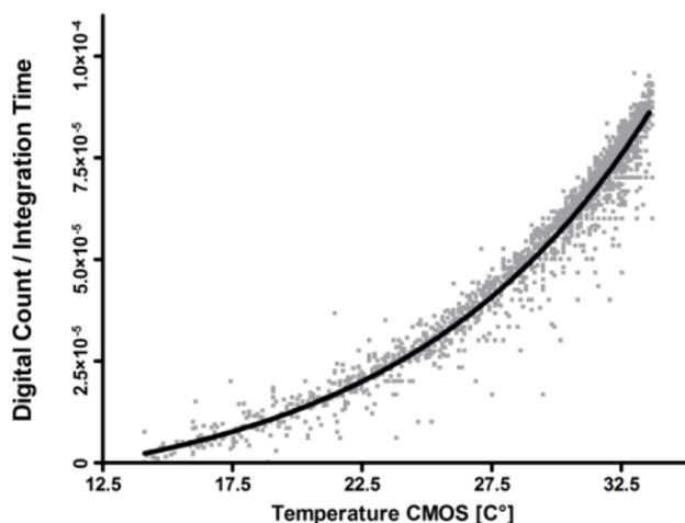
Fig. 3. Exponential regression of dark current dependency to raising detector temperature shown for Pixel 4 of the air unit's STS microspectrometer (n = 1854,  $R^2 = 0.9586$ ). Data was fitted with an exponent function  $y=a+b*e^{cx}$ .
