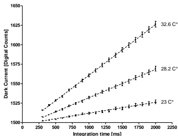
Fig. 2. Linear regression of dark current at three different detector temperatures and changing integration time. Dots and whiskers are mean values and standard deviations respectively for all spectral bands ( $n = 256$ ).
