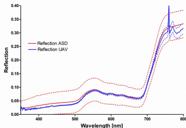
Fig. 5. Reflection over grassland measured by ASD field spec (n = 75) and UAV spectrometer (n = 8). Standard deviation is indicated by the dotted lines. Standard deviation on the other targets (wheat and soil) was similar high in ASD measurements and low in the UAV measurements.
